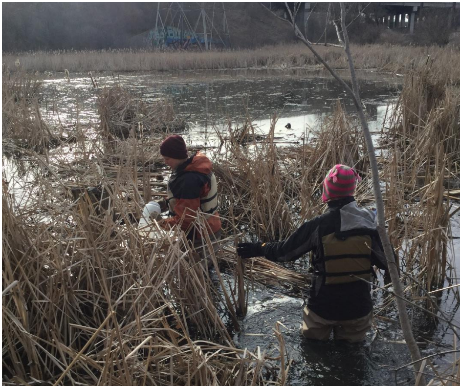
Figure 3. Collecting a water quality grab sample from Kasota Pond North.
