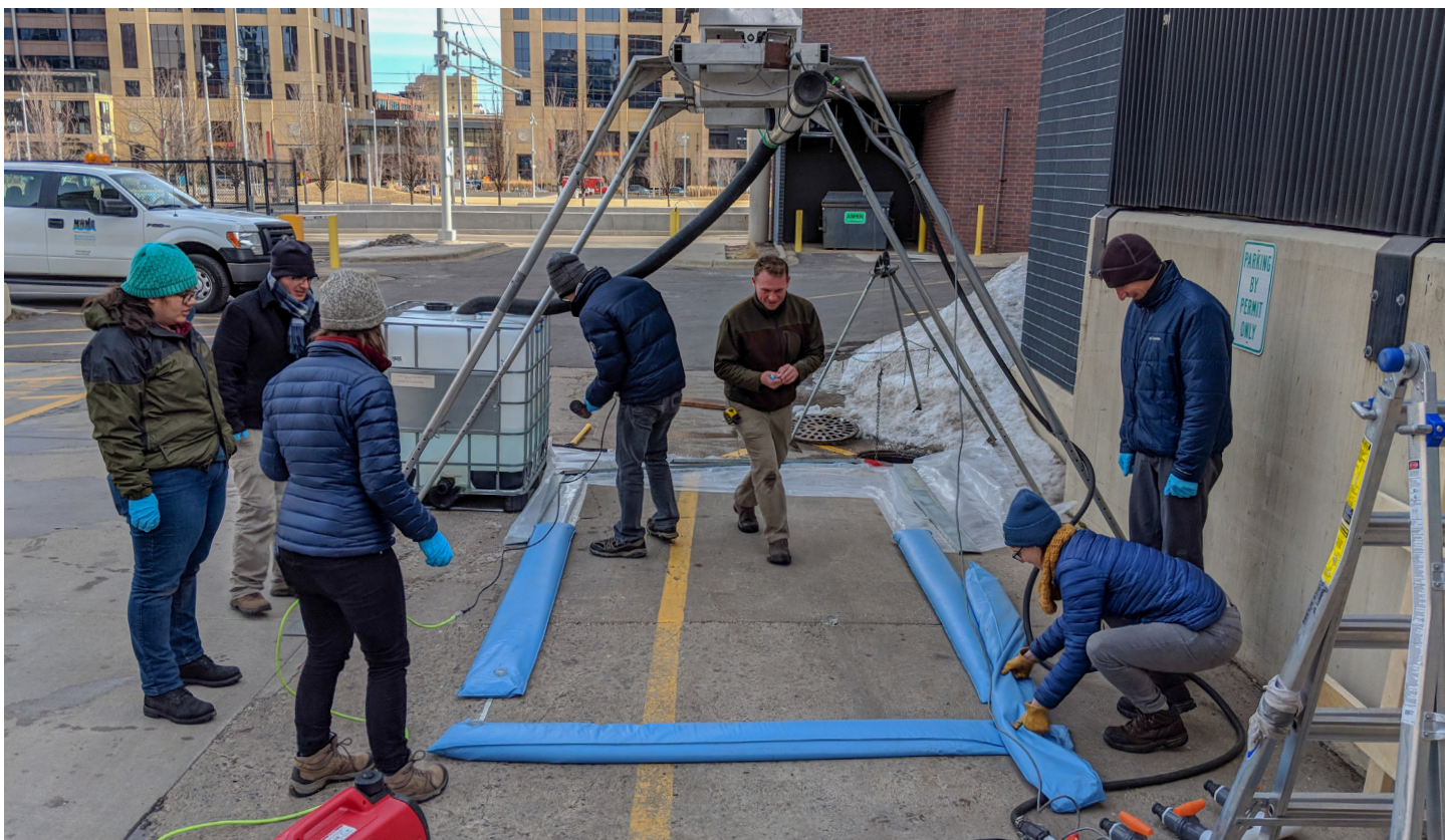
Figure 6. MWMO staff and University of Minnesota researchers prepare a rain simulator test to collect water quality samples of runoff from a downtown Minneapolis parking lot on March 23, 2018. The team's work is documented in a new report, "Analysis of Runoff from Impervious Surfaces in Downtown Minneapolis."
