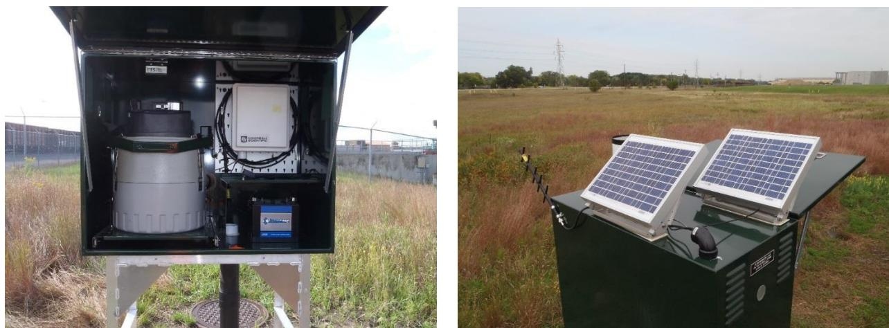
**Figure 4.** Example of a typical MWMO stormwater monitoring site cabinet set up including automated sampling and real-time monitoring equipment.
