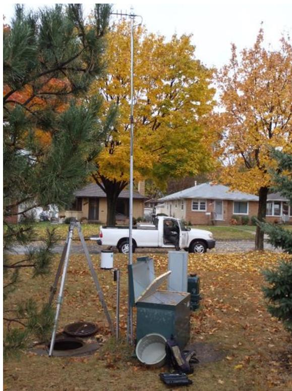
**Figure 15.** Monitoring equipment and access manhole at the 10SA stormwater site
