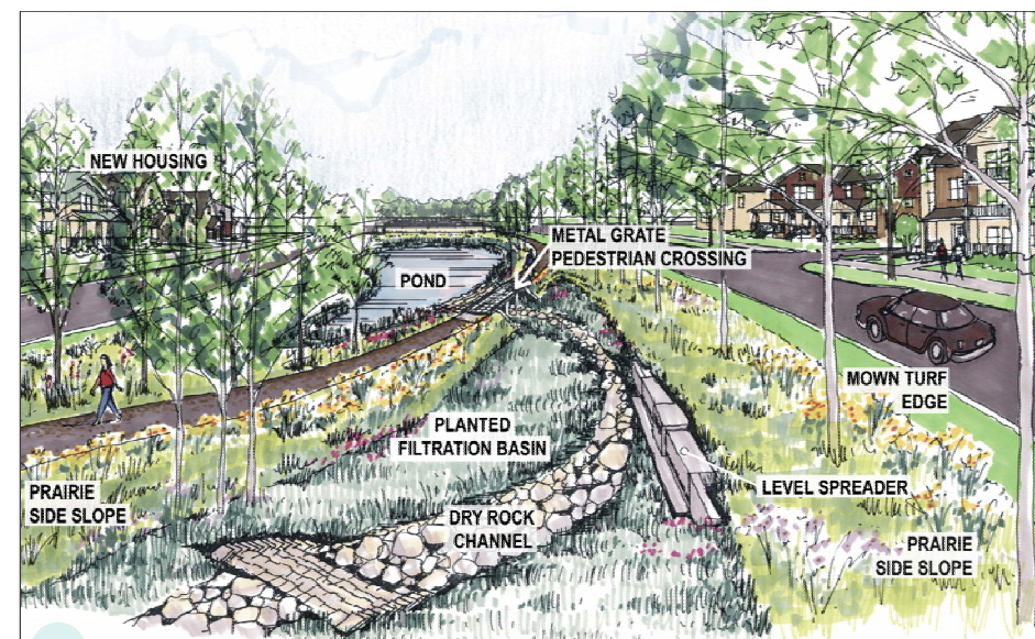
A Looking north, toward wet basin in distance. Filtration basins, with rock channel, in foreground.
