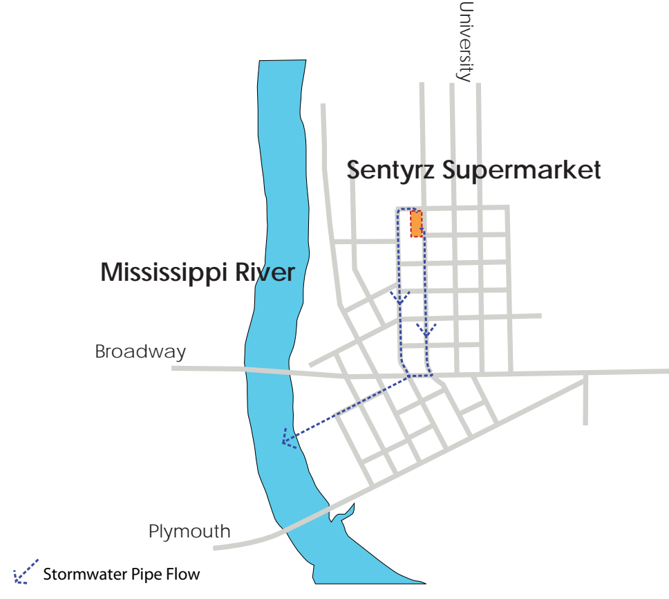
Path of Stormwater Through Stormdrains to the Mississippi River
