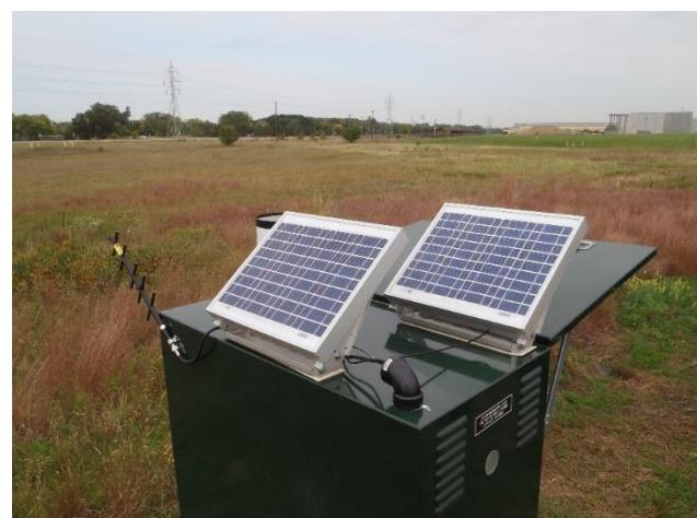
**Figure 4.** Example of a typical MWMO stormwater monitoring site cabinet set up including automated sampling and real-time monitoring equipment.
