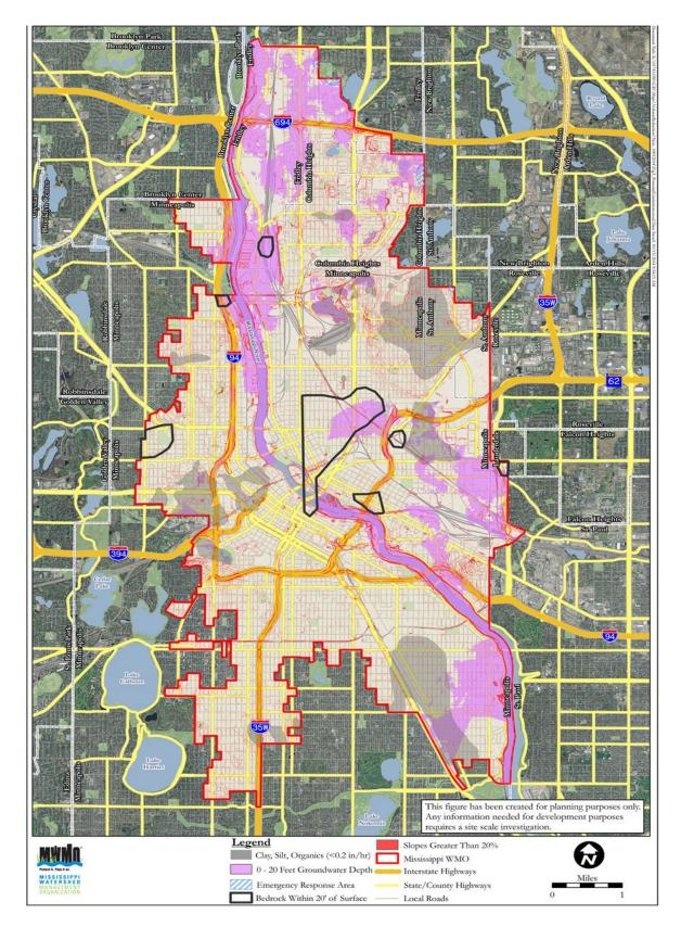
Figure 2: Potential Limitations to Infiltration
