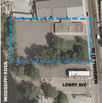
ABOVE: The location of the new MWMO headquarters in Northeast Minneapolis is shown in blue. This was the former location of the International Brotherhood of Electrical Workers (IBEW) where nearly 75% of the 1.29 acre site was covered with hard surfaces (roof and parking lot). Hard surfaces do not absorb water, which means that all the rain and snowmelt wash off directly into the adjacent river.
